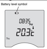
The batteries need changing when the battery level symbol appears (2 LR03 or AAA 1.5V alkaline batteries).
