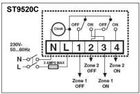
Just replace existing timer, fits directly onto many other timer backplates. No power supply required to cylinder sensor.
