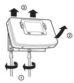
To remove the unit from the wall-plate, slacken the two securing screws at the bottom of the ST9400 and hinge the unit up to separate the two halves.
