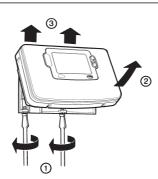
To remove the unit from the wall-plate, slacken the two securing screws at the bottom of the ST9100 and hinge the unit up to separate the two halves.
