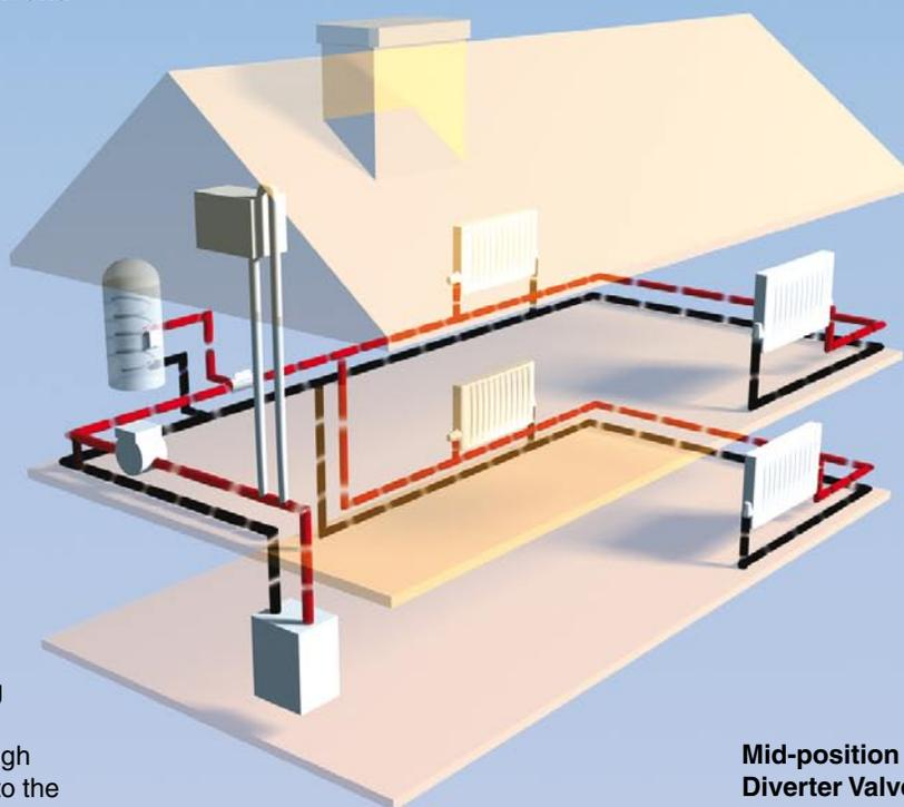
This simplified illustration shows the principal components in your heating system. Water heated in the boiler is circulated through the pipework by the pump, to the radiators and storage cylinder under the control of the zone valves.
