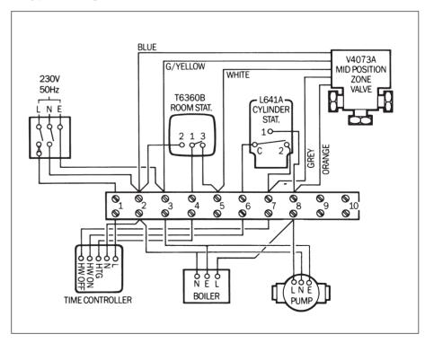
Note: It is recommended that the 10 way Junction Box or Sundial Wiring Centre should be used to ensure first time, fault free wiring.
