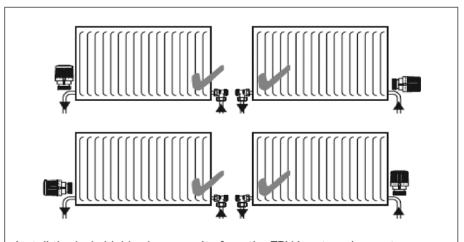
Install the lockshield valve opposite from the TRV in a two-pipe system.
