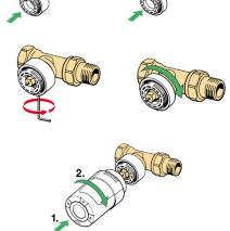
4. Activate Installation Mode to fix *living eco*® correctly onto the valve:
