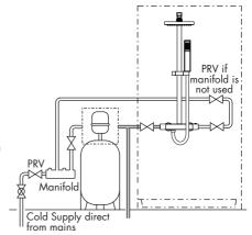
It is recommended that the cold supply be taken from one of the outlets of the manifold directly to the shower as an independent supply.
