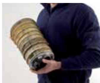
Heat exchanger damaged by system debris and pollutants
