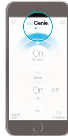
1. **Slide through zones** by swiping left or right in the highlighted area.
