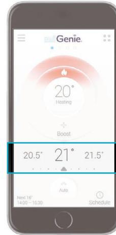
2. To change the temperature of a room or zone, simply slide **LEFT** or **RIGHT** until the desired temperature appears in the middle.
