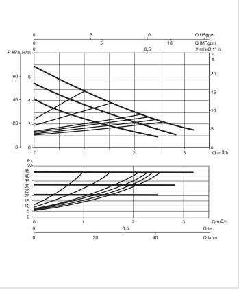
The performance curves are based on kinematic viscosity values = 1 mm<sup>2</sup>/s and density equal to 1000 kg/m<sup>3</sup>. Curve tolerance according to ISO 9906.
