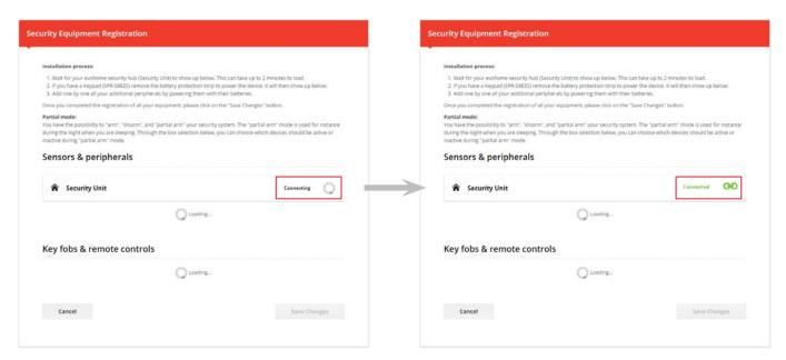
Now register each accessory by powering each one up one after the other. Details for the accessories are explained in this section or in the supplied installation guide for that accessory
