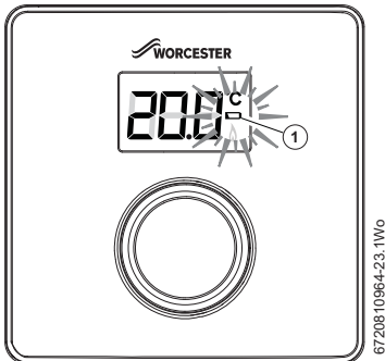
Fig. 22 Low battery indication
