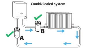
In both diagrams, position **A** is best practice while **B** is suitable. N.B. We firmly recommend MagnaClean Micro is installed and serviced by a qualified heating engineer.
