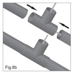
8. Thread the Trace Heater Cable through the bung (from the narrow end) and push the bung into the T piece to seal the pipe. You may require a sealant at the cable exit (see Fig.9a and b).
