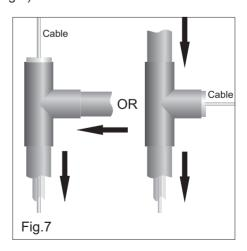
7. Pass the Trace Heater Cable through the selected opening in the T Piece and fit the T Piece to the Condensate Drain Pipe and fix using the appropriate adhesive (see Fig.8a and b)
