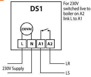
LS & LR ARE NORMALLY THE ROOM THERMOSTAT CONNECTIONS
