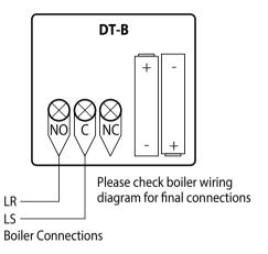
Note: LS & LR may be labelled differently but they are normally the boiler's room thermostat connections.
