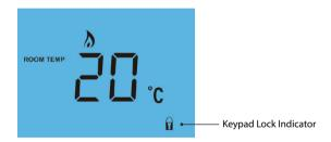
The keypad lock indicator is only visible when the lock is active.
