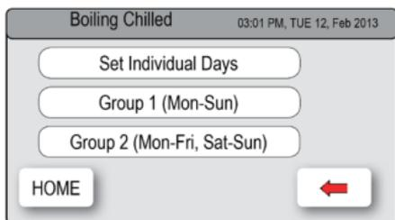
On/Off mode allows the user to turn the unit on or off at a specific time.
