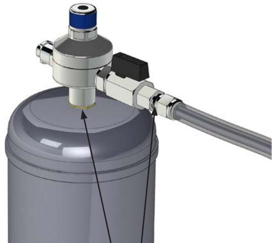
Test for leaks at these two points
