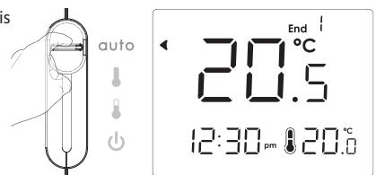
**COMFORT:** Permanent comfort mode. The unit is controlling continuously to the comfort temperature setpoint. The default temperature setting is 20°C (68°F). Refer to section temperatures setting to change the value page 2.
