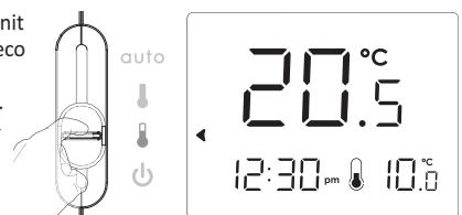
**STANDBY:** Permanent standby mode with frost protection. The unit is controlling continuously at the frost protection temperature factory set. i.e 8°C.
