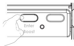
BOOST is cancelled by any press of button, movement of dial or slider. When BOOST is running the time and day disappear. The minute array will count down from 60 – 0 to indicate time left in BOOST mode.
