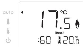
BOOST will work from any running mode. BOOST is entered by pressing Enter/Boost button.
