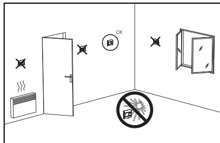
**Important:** The thermostat measures the temperature of the place where it is installed. It does not take into account the temperature differences that may exist between different locations in the house if the temperature is not uniform.
