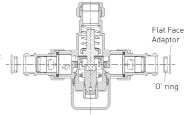
3. Insert the flat face adaptor assembly into the hot and cold inlet ports.
