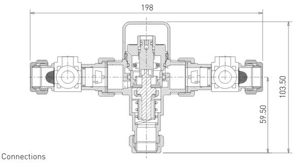
Inlet: 15mm compression Outlet: 15mm compression
