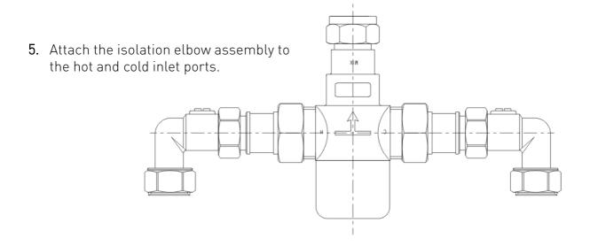
$\begin{tabular}{ll} \textbf{Note:} Check all joints and connections are sealed from leakage. \end{tabular}$
