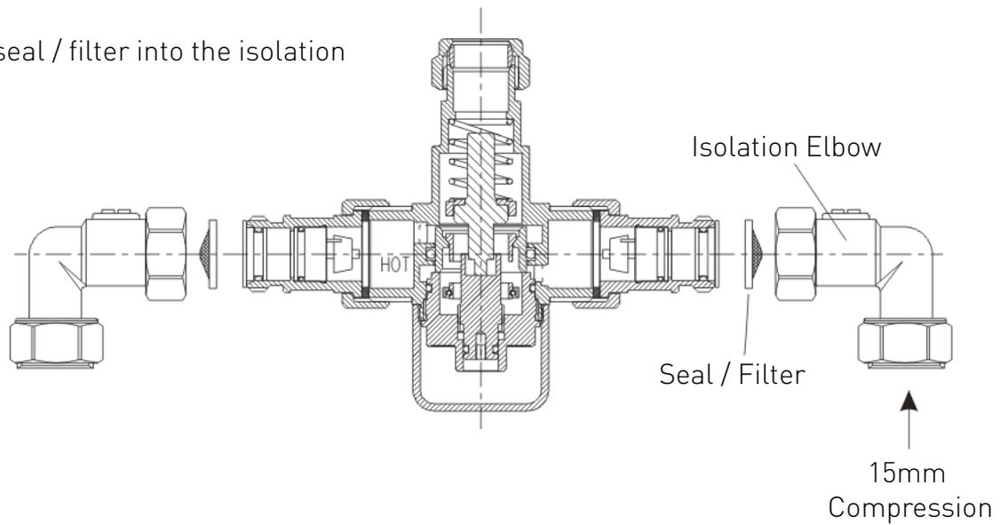
5. Attach the isolation elbow assembly to the hot and cold inlet ports.
