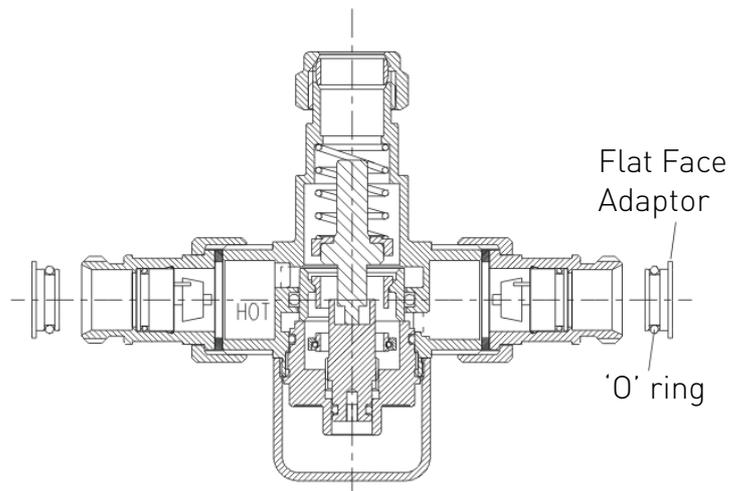
3. Insert the flat face adaptor assembly into the hot and cold inlet ports.
