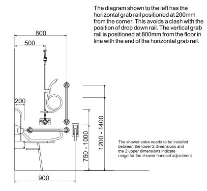
Shower controls shown must fall within the 750mm to 1000mm above the floor requirement. Positioning the centre of the Shower Diverter at the 1000mm height sets the thermostatic mixer valve at a height such that it does not interfere with the rails. Adjustability of the shower handset is greater than the required heights but should be operable between the 1200mm and 1400mm heights shown.
