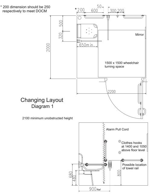
N.B. The above diagram is to the dimensions given in Approved Document M and will give a clash between the horizontal and vertical grab rails and the drop down rail. Either the grab rails may be moved or the drop down rail itself (choice is left to the installer) but it would be recommended to move the horizontal grab rail to start at 200mm and not 250mm as directed by the Doc M guide dimensions. The drop down rail maintains its position of 900mm from the corner.
