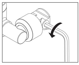
4. Turn the flow of water on by turning the flow handle to the 'On' position.
