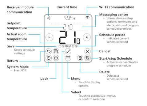
**Note:** To save power, the screen will dim and enter idle mode 45 seconds after the last button touch. The screen will light up when you touch any button.
