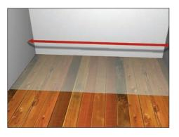
Measure the required overall length of the shower area with a tape measure. We would not recommend an area less than 1250mm in length because this would not allow a wide enough opening to get in and out of the shower easily.
