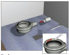
Note: Make sure all pipes and drainage parts are clean at all times using solvent waste pipe cleaner prior to connection.
