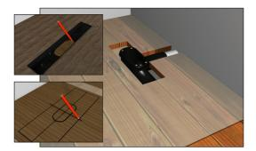
Measure the shower drain base position on the floor and mark this onto the relevant flooring. The size of the cut-out needs to be 315mm x 90mm. Make sure that the drain's centre is in the middle of the cut-out.
