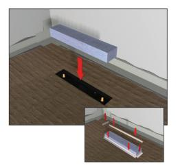
Place the disposable tiling aid into the shower drain hole on the shower tray. The tiling aid provides the edge that needs to be tiled up to whilst protecting the drain from debris. At this stage we recommend fitting tile trim to create a clean finished edge for the waste cover.
