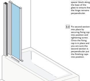
3.2 Place second section of screen onto the bottom hinge of the first section with spacer block along the base of the glass to ensure that the hinge remains perpendicular.
