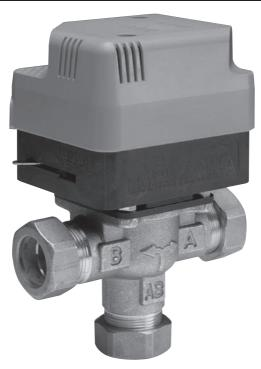
The Z322 mid-position valve has been designed to control the water circulation in fully pumped systems, which employ a single pump for both hot water and central heating circuits by diverting the flow to either or both simultaneously using a single valve.
