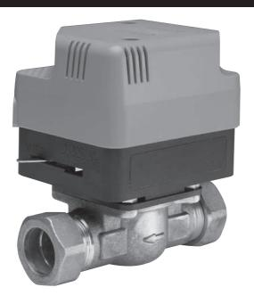
The Z222 valve with auxiliary switch has been designed to control the water circulation in fully pumped systems, which employ a single pump for both hot water and central heating circuits by allowing the flow to either or both circuits using separate valves.
