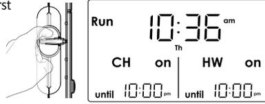
Auto: Automatic mode. The unit is controlling to the programming that have been selected (refer to "Programming" section page 2).
