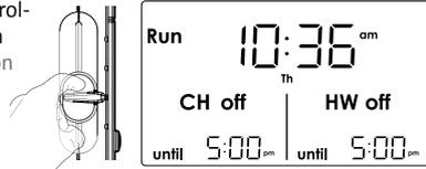
Off: Permanent Off mode. The system stays Off permanently. The boost mode can be still used.
