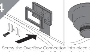
Screw the Overflow Connection into place and connect to the waste body. Carefully turn the sink upside-down.
