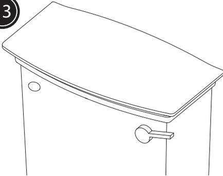
Fit the lever and place the lid onto the cistern, use cistern blanking plug to cover unuse hole.
