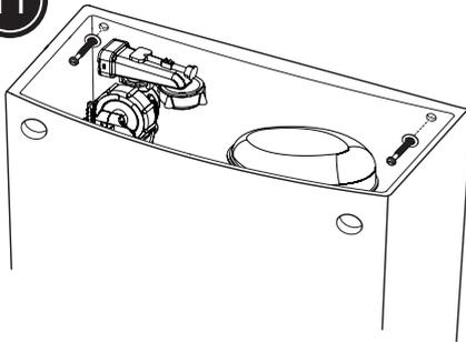
Fix the cistern to the wall with screws and washers (not supplied). Ensure the cistern is not pulled backwards, as the seal with the pan might broke.
