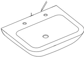
1. Decide on the final position of the basin. Install suitable bottons onto the wall cavity to support the weight of the basin if required.
