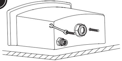
Insert fixing bolts through the holes in the cistern, using the rubber and large metal washer.
