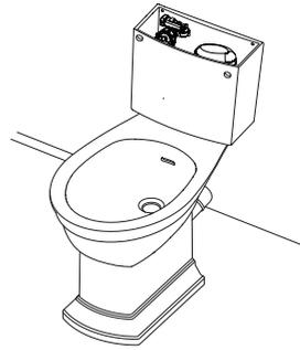
Return the pan to the desired location, make the plumbing connections and ensure that they are water tight. Ensure the pipework is flushed prior to connecting the cistern.
