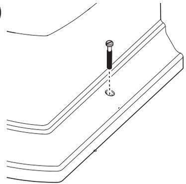
Insert screws at the base of the toilet to fix the pan to the floor using the washers provided. Do not overtighten.
