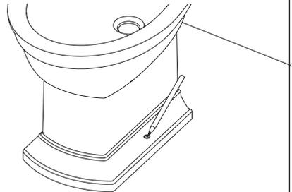
Draw a line around the base of the pan to clearly mark the position and mark the position of the screw holes.
