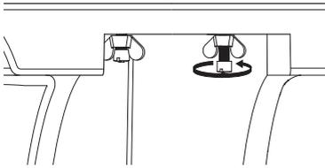
Fit the washers and wing nuts to the underside of the cistern and tighten the nuts.
