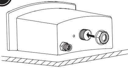
Position the cistern on its back. Assemble and insert the flush mechanism.
