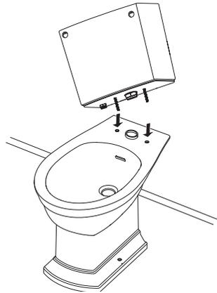
Lift the cistern onto the pan so the connecting bolt fit through the holes.
