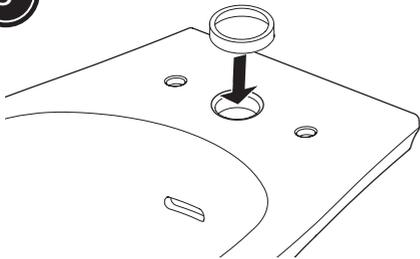
Place the large rubber gasket into the flush entrance of the pan.
