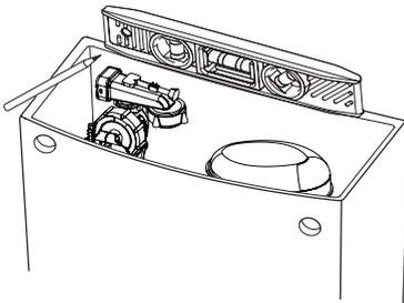
Ensure the cistern is level by placing spirit level along the back against the wall. Mark off the fixing holes through the back of the cistern.
