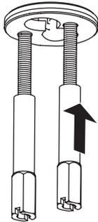
Slide the metal plate onto the threaded rods under the basin and secure the fixing base to the basin by tightening the fixing nuts onto the fixing rods. Ensure the fixing nuts are tightened fully by using a suitable spanner.
