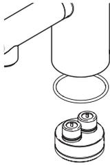
Push the mixer body onto the fixing base ensuring the rubber 'O' ring is fitted into the groove in the bottom of the mixer body. Ensure the mixer body is fitted correctly and tighten the grub screws fully to secure the mixer body in position.
