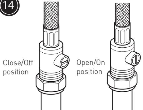
Connect the cold water supply. Turn on water supply at the isolation valve and check for leaks.
