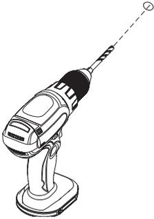
Drill fixing holes for cisten/pan through the marks on the wall/floor. Use wall plugs according to wall/ floor surface.
