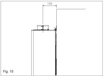
Fit the appropriate flashing plate to the roof and insert the vertical flue terminal through the flashing plate from the outside, ensuring that the collar on the flue terminal fits over the flashing. The fixing holes for the wall-mounting bracket should now be drilled and plugged, an 'appropriate type and quantity of fixing should be used to ensure that the bracket is mounted securely. Once the bracket has been secured to the wall, mount the appliance onto the bracket.
