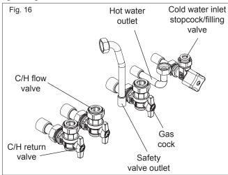
**4.6.1 GAS (fig. 16)** The appliance is supplied with a 22mm service valve, connect a 22mm pipe to the inlet of the valve and tighten both nuts. NOTE
