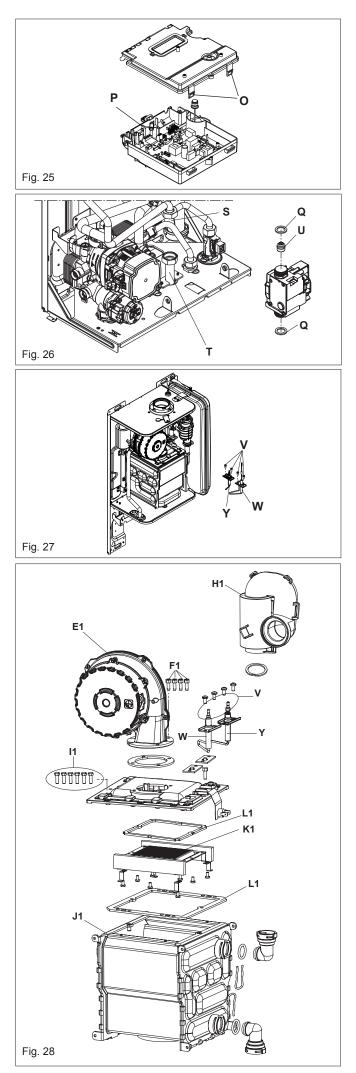
Disconnect the flow locking pin (M1), return locking pin (N1)on the heat exchanger. Locate and remove the 4-screws that secure the heat exchanger to the combustion chamber (O1). Move the heat exchanger and disconnect it from the flue collector (P1). The heat exchanger can now be lifted up and withdrawn from the appliance.
