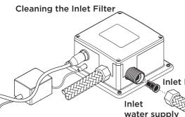
Before carrying out any maintenance. turn off the mains water supply and close any isolating valves.
