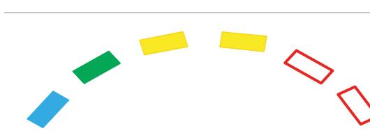
The same behavior applies to the two subsequent (yellow) LEDs, until the set temperature of 55°C is reached (all LEDs stop blinking).
