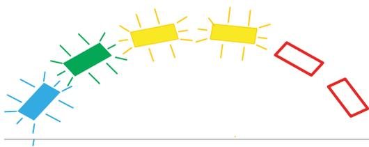
The device is firstly turned on. Pressing the [+] button 4 times sets the desired temperature at 55°C (the first 4 LEDs from the left start blinking).
