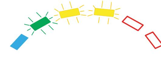
The radiator starts heating. When its temperature reaches 40°C the first (blue) LED stops blinking and remains lit.
