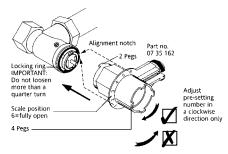
i.Remove the thermostatic or wheelhead and loosen the locking ring.
