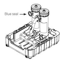
**5** Attach the valves to the inlets on the *RapidFlush* filter. Fit tri-clamps over the pair of flanges, seal and tighten screw. Ensure the hose containing the drain off is attached to the bottom right inlet.
