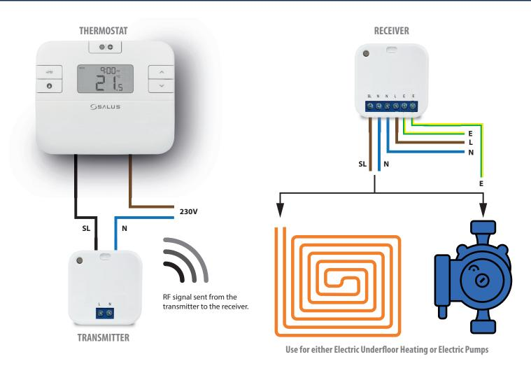
In the example above we show a thermostat connected to the SALUS Main Switch transmitter. When the thermostat calls for heat it sends an RF signal to the receiver which then turns on either the Electric Underfloor heating or the Electric pump depending on the system.
