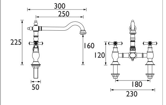
Flow Rates (I/min) System Pressure (bar) 0.2 0.5 5 2 3 K BRSNK BN (mixed) 15.7 24.8 35.1 49.6 60.8 78.5 TECHNICAL BR DATA S D12
