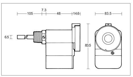
L6188B2000 TP\* Controller, setting 25 to 95°C, Diff. 4°C. Without wiring terminal cover
