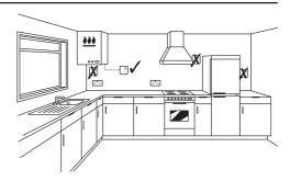
For best performance, install in an open space. Leave at least 30cm distance from any metal objects including wall boxes and boiler housing. Do not mount on metal wall boxes.
