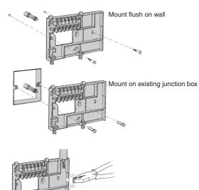
Breakout tabs accommodate surface wiring if needed
