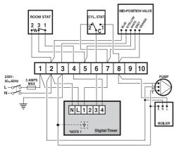
**Note 1:** This is a Class II device (i.e., double insulated). A parking terminal is available for earth wiring if required.
