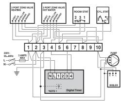
**Note 3:** Gravity circulation hot-water systems should be fitted with a suitable hot-water control valve as shown in Plan C on page 19. If this valve is not installed, configure this device as a Mini-Programmer (see page 24).
