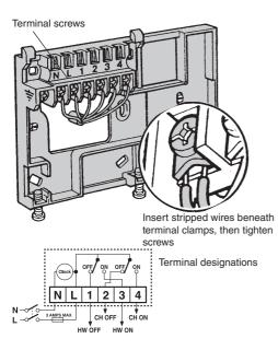
Connect wiring from your heating and hot water system to the Digital Timer terminal screws as shown at left. See wiring diagrams on pages 18-20.
