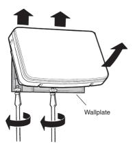
Use a screwdriver to loosen screws and separate the Digital Timer from the wall bracket as shown at left.
