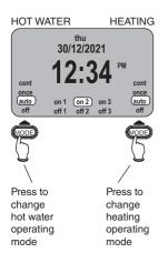
Press the *MODE* button repeatedly to select an operating mode. You can set the Hot Water and Heating modes separately, by pressing the appropriate button as shown at left. Both work the same way:
