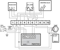
**Note 3:** Gravity circulation hot-water systems should be fitted with a suitable hot-water control valve as shown in Plan C above. If this valve is not installed, configure this device as a Mini-Programmer.
