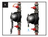
Close both isolation valves, open the air vent, then open the drain valve and drain the unit.
