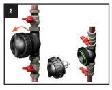
Re-insert drain valve, unscrew locking collar and remove the filter bowl and core.
