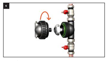
Locate the filter bowl and core into place by tightening the locking collar, making sure the air vent is positioned at the top.
