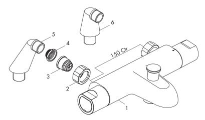
Note: The deck mounting legs are supplied complete with retaining nuts.
