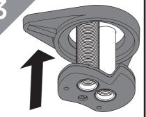
Feed the base through the sink hole from the top.
