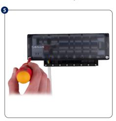
Make sure that all the wires are properly connected, mount top cover and power up the control box - the red power indicator LED will be illuminated.
