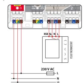
Connecting a 230 V thermostat to the CB500 control box (e.g. SQ610)
