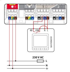
Connecting ON/OFF battery-powered thermostat with voltage-free COM / NO output contacts (e.g. 091FL, RT310, RT510)
