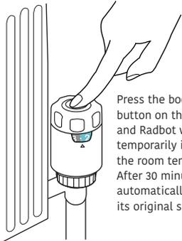
Press the boost button on the top and Radbot will temporarily increase the room temperature. After 30 minutes it will automatically return to its original settings.
