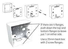
3. Route the wires through the back of the wall plate. Fit the wires to the wall-plate in accordance with the relevant diagram and in accordance with I.E.E. regulations.
